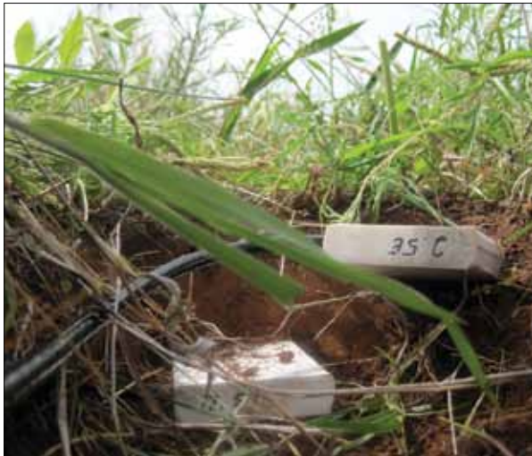
Probes are buried in the ground at different depths to estimate soil moisture content, but they only measure moisture within several inches of the instrument. (Courtesy J. Braun)
