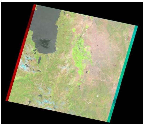
**Figure 6-1. Edge Striping in Visible GeoTIFF having SWIR Band.**
