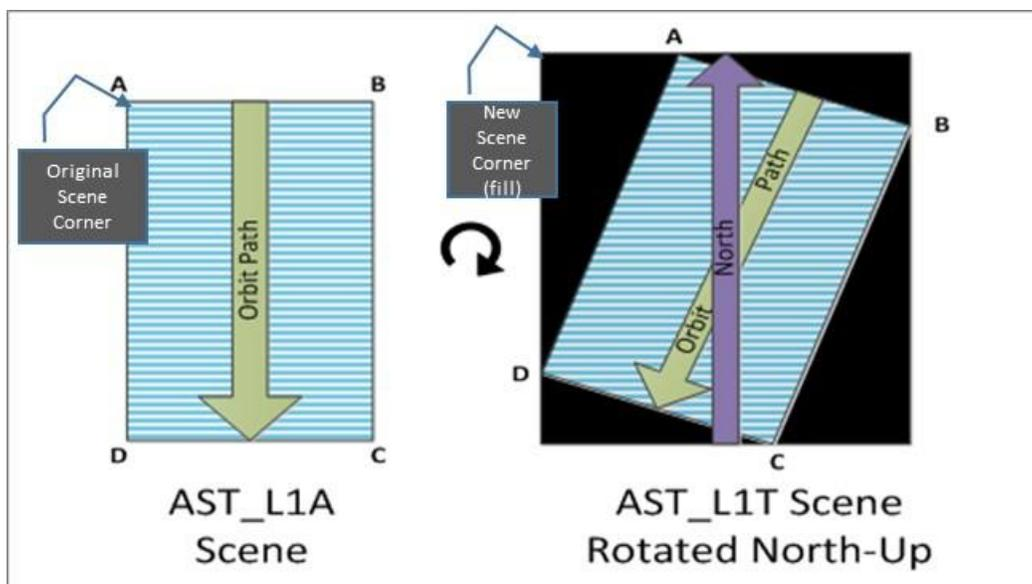
**Figure 2-2. AST\_L1A Image Rotated North-Up in AST\_L1T Product.**
