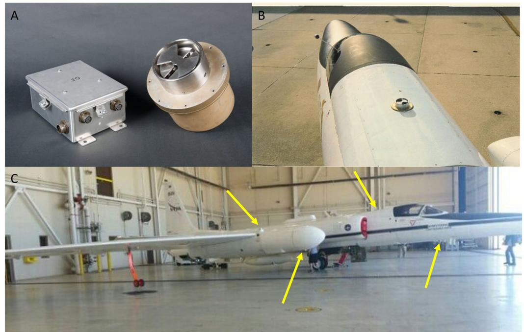
**Figure 1.** Images of the Lightning Instrument Package field mills, data box (panel A), and locations on the ER-2 Aircraft (panels B, C). Not shown are the three mills on the left wing, two of them mirroring the location on the right wing, and a third on the lower aft part of the left superpod.
