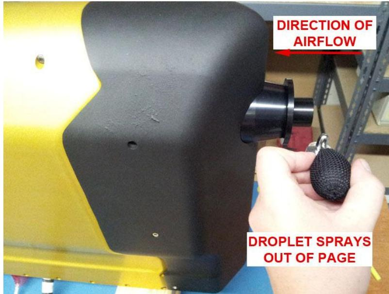
**Figure 3.4.6.** Spray droplet atomizer across Hawkeye inflow, perpendicular to direction of airflow into the instrument.
