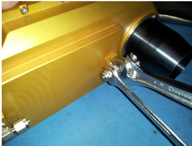
**Figure 3.1.9:** Use the 1/2" wrench on the nut most near the body to hold fitting. Use the 7/16" wrench on the cap. **DO NOT BREAK THE SEAL ON FITTING WHEN REMOVING CAP.**
