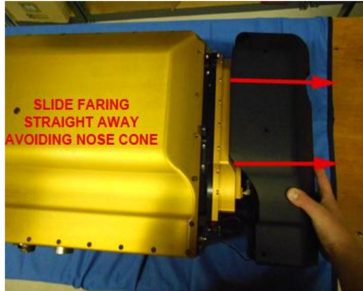
**Figure 3.1.6.** Remove the Front Fairing by sliding it a few inches straight forward.
