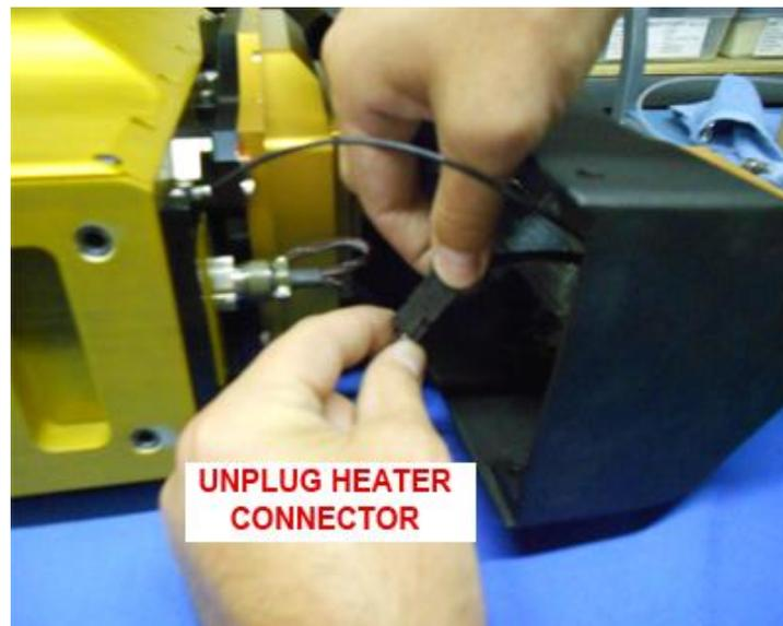
**Figure 3.1.7.** Prior to complete removal of the Front Fairing, unplug the heater connector.
