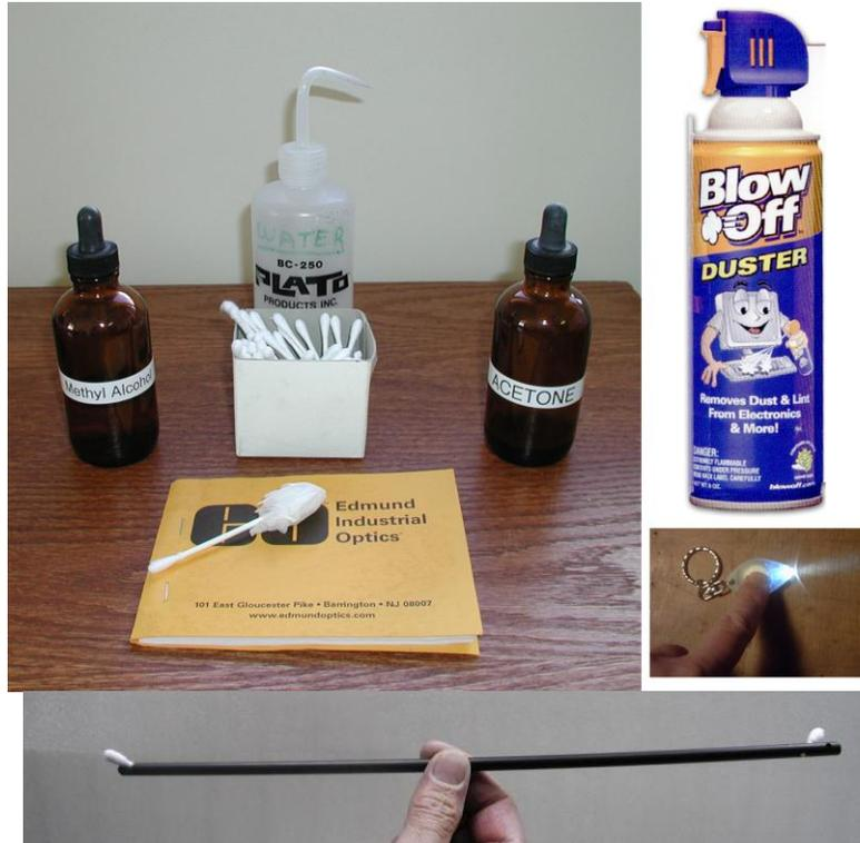
**Figure 3.2.2.** Items needed for cleaning the Hawkeye optical windows.
