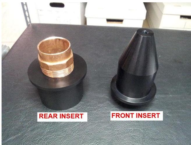
**Figure 3.4.3.** Hawkeye Front and Rear Inserts for atomizer setup.
