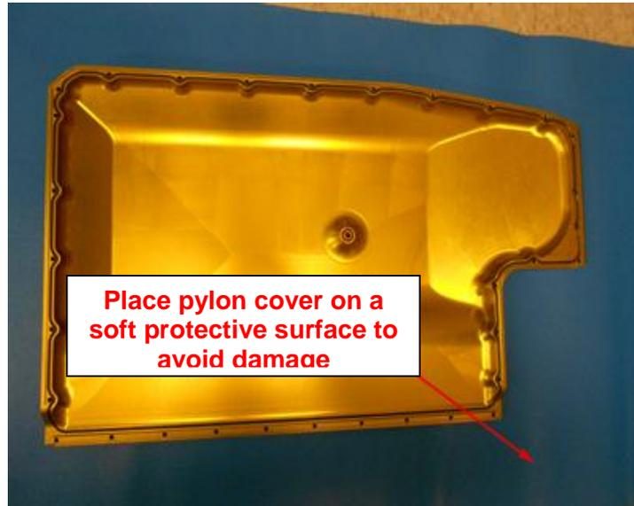
**Figure 3.3.5.** Place pylon cover on static mat.
