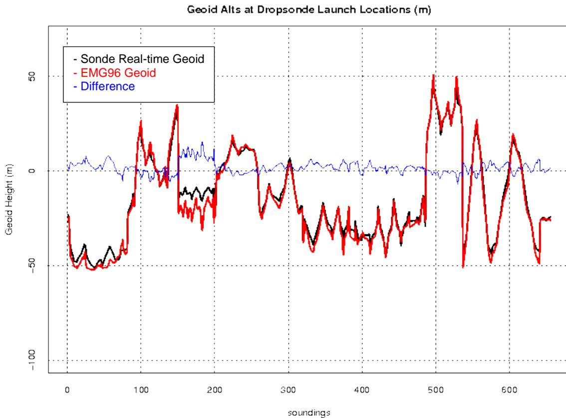
**Figure 4 Sonde GPS and EMG96 Geoid Altitudes and difference.** Black line shows dropsonde geoid values originally contained in real-time dropsonde GPS altitudes. Red line shows the geoid measurements from the EMG96 which replaced the dropsonde geoid values.
