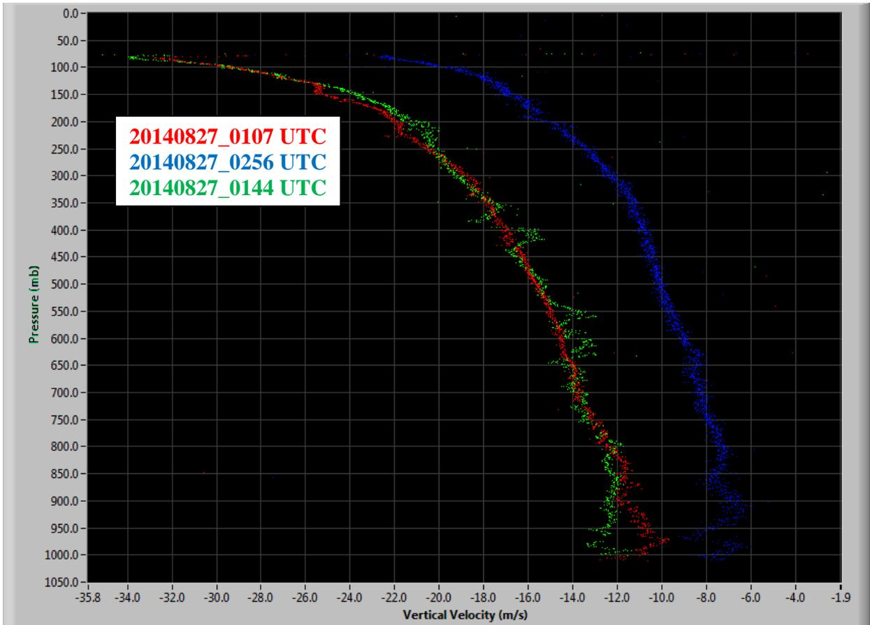
**Figure 5 Profiles of typical vertical fall rates and large parachute fall rate.**
