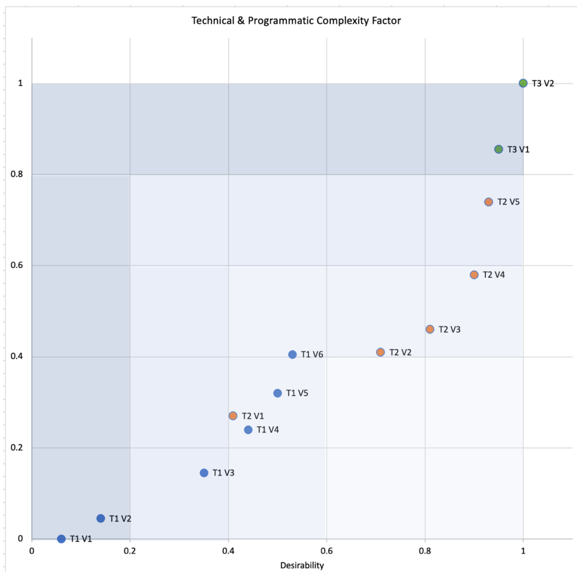
Figure 6-3. Combined Technical and Programmatic complexity of each architecture relative to the architecture desirability. With this chart we conclude that Architecture T2V3 is the optimal choice because it is mathematically closer to the point of minimum complexity and maximum desirability.
