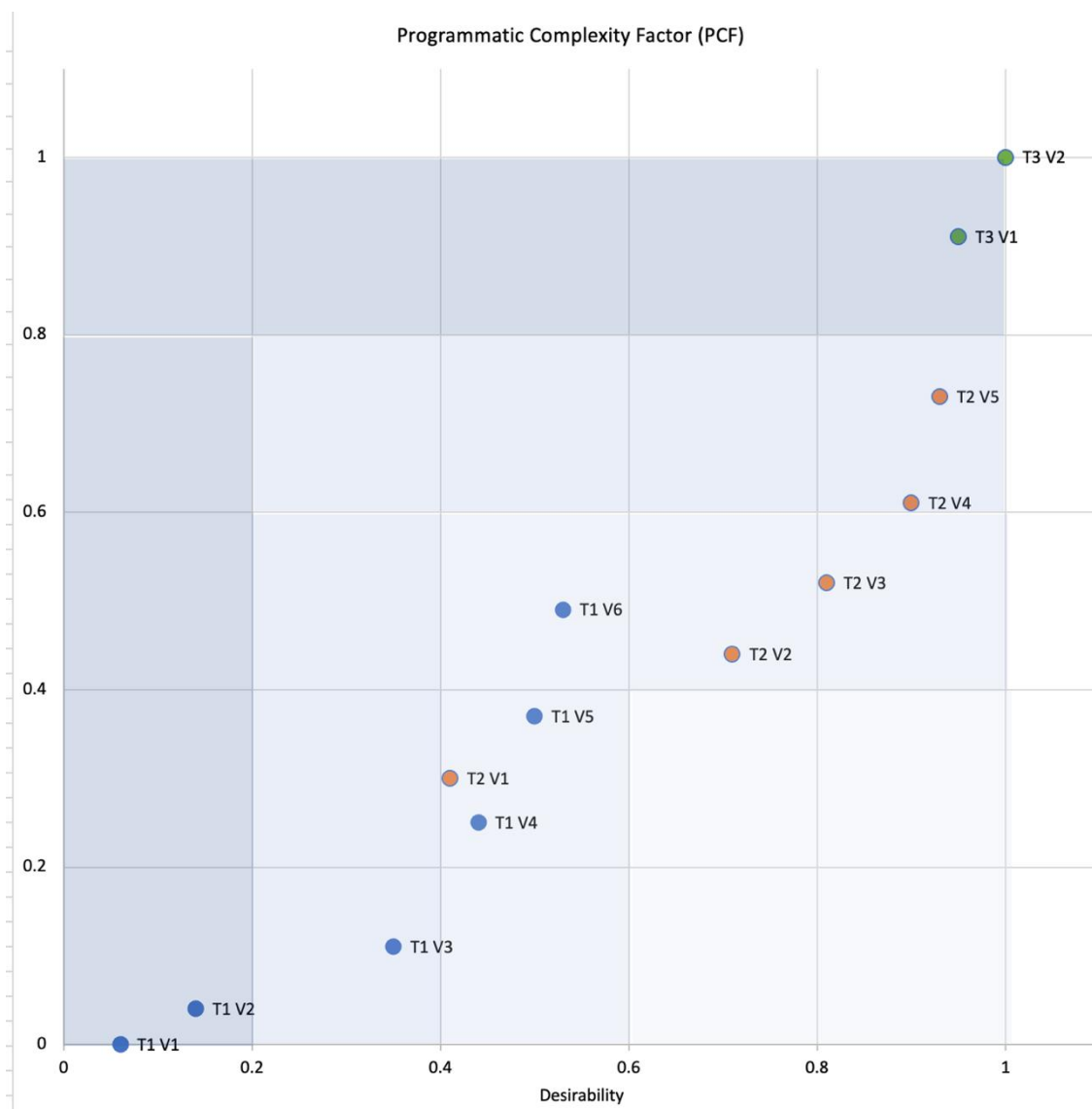
Figure 6-2. Programmatic complexity of each architecture relative to the architecture desirability. This chart suggests that Architecture T2V2 is the optimal choice from a programmatic perspective because it is mathematically closer to the point of minimum complexity and maximum desirability.
